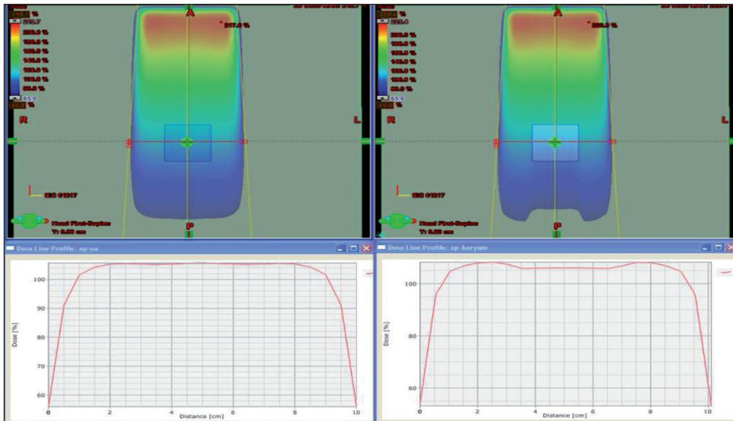
FIGURE 3: Dose distribution profiles of lateral axis obtained with contrast and uncontrasted cubic phantom.
