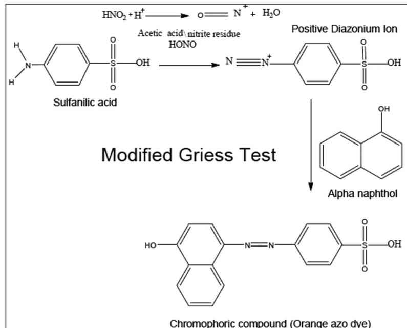
**FIGURE 1:** The chemical reaction for the Modified Griess Test (The orange color is caused when the nitrites are introduced to acetic acid and heated to form nitrous acid. The nitrous acid then forms a diazonium compound with sulfanilic acid, and this compound then couples with the alpha-naphthol to produce the orange azo dye).
