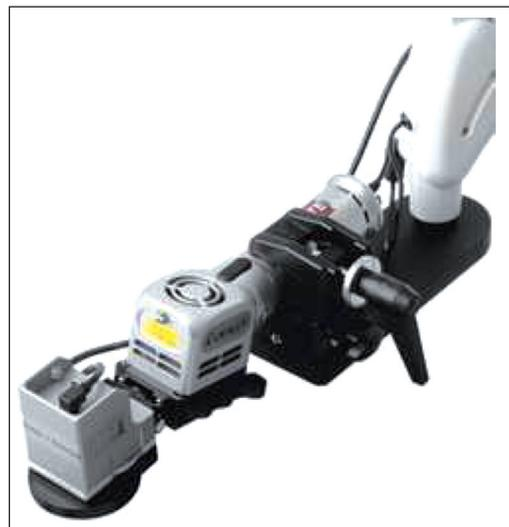
**FIGURE 3:** Crime-lite 82S with 5MP IR sensitive camera.
