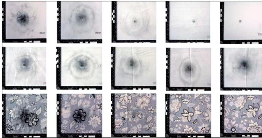
**FIGURE 8:** IR camera photographs of original fired grey fabrics (top), colored fabrics (middle), and the patterned samples (bottom). Examples of unknowns (middle, from left to right: orange, maroon, navy, black, grey all fired at 10 inches) while known distances of top and bottom images are in order from left to right: contact, 6 inches, 12 inches, 24 inches, 36 inches for grey and patterned fabrics.
