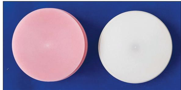
FIGURE 5: Computer-aided design/computer-aided manufacturing polymethyl methacrylate and polyether ether ketone discs used study.
