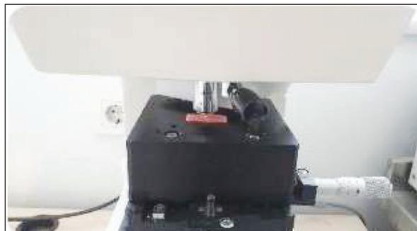
FIGURE 9: Hardness measurement from test specimens.
