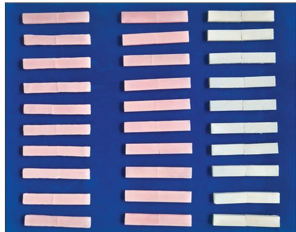
FIGURE 2: TC (+) specimens for flexural strength and elastic modulus tests.
