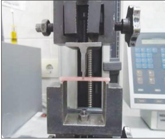
FIGURE 7: Three-point bending test.
