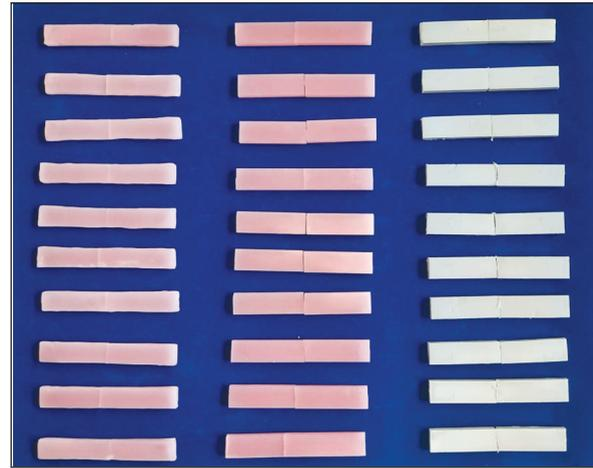
FIGURE 1: TC (-) specimens for flexural strength and elastic modulus tests.
