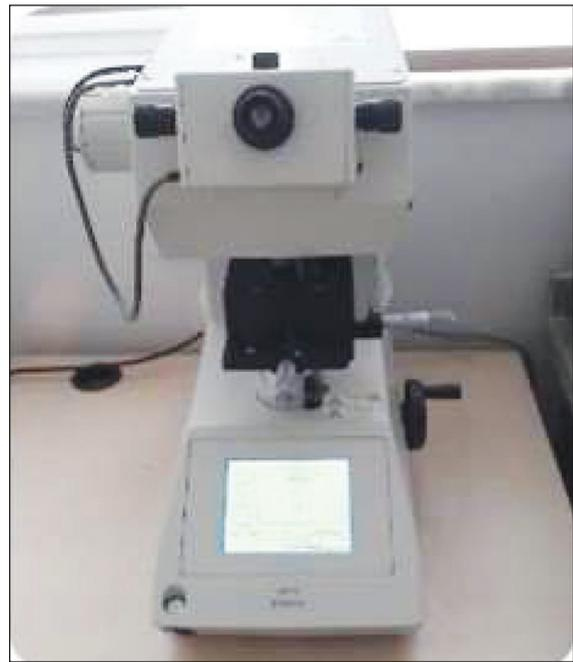
FIGURE 8: Vickers micro hardness test device used this study.
